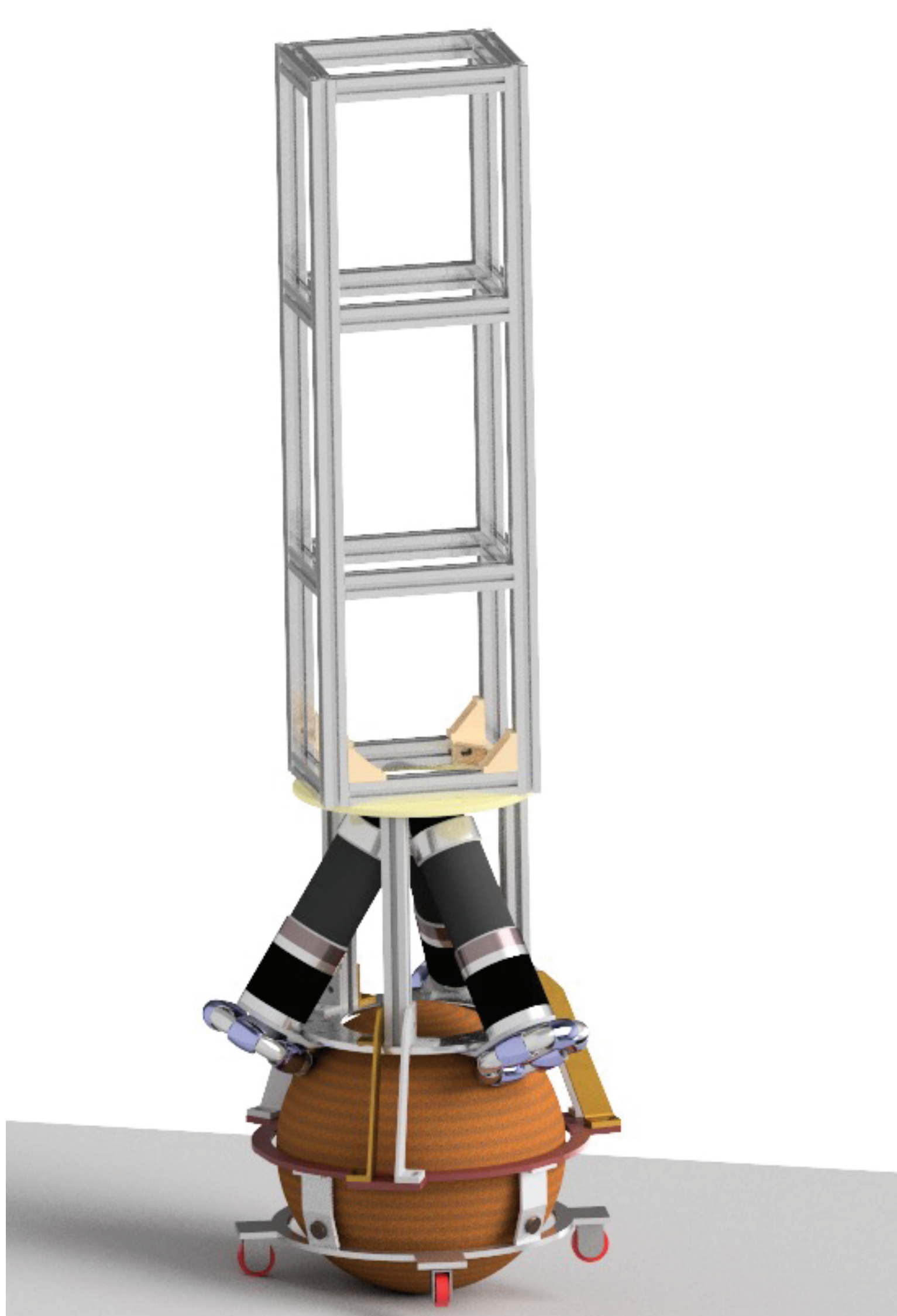
Ballbot bearing frame structure
